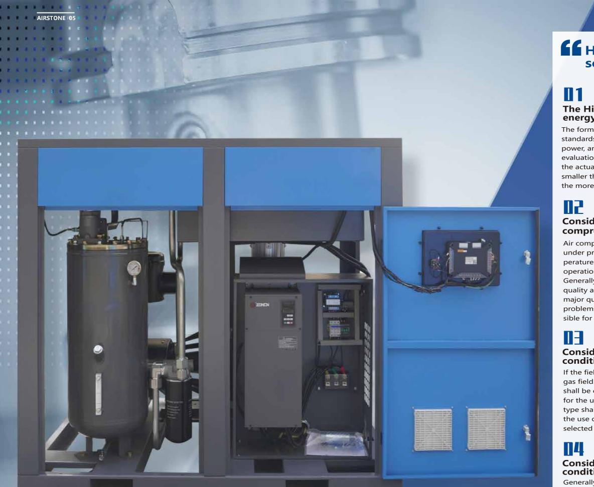
Generally, the compressed air produced by the air compressor contains a certain amount of lubricating oil and water. In some cases, oil and water are prohibited. At this time, attention should be paid to choose oil free compressor
